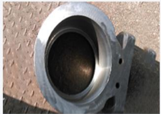
bearing housing for electrical loco DIN1782 material
